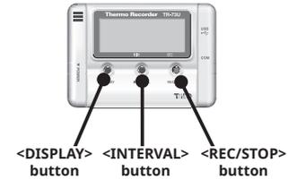
**DISPLAY :** Pressing this button will change the LCD Display Mode.
