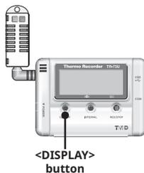
2. If the LCD display shows three channels' readings alternatively, it will show one channel as a fixed display by pressing the button. By pressing the button again, the LCD display pattern will be set for displaying three channels alternatively. If the display has been set for a fixed channel, with each pressing of the button the channel display will change.
