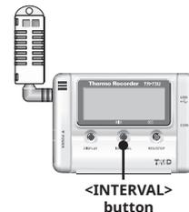
1. Press in the <INTERVAL> button on the front of the device until the recording interval appears in the display.
