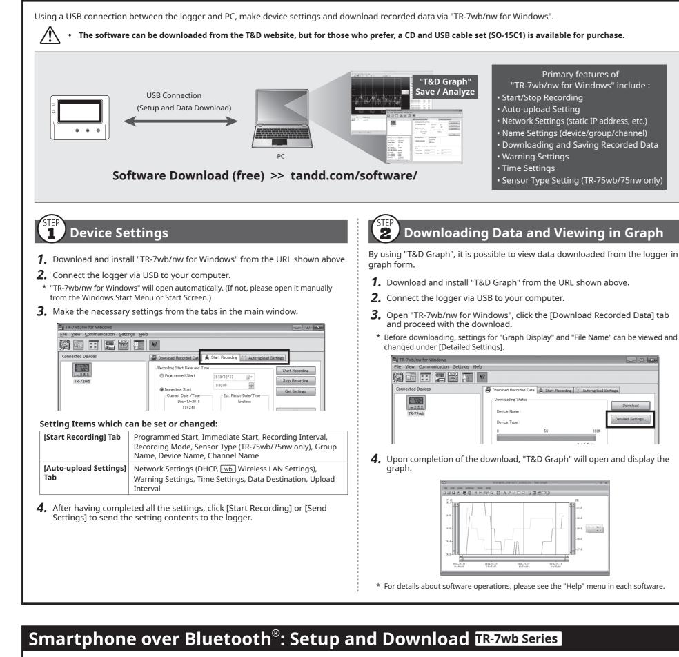
By using the "T&D Thermo" App with wb, it is possible to make device settings, download recorded data, and view recorded data directly from your smartphone or tablet via Bluetooth. The app supports Android OS and iOS.
