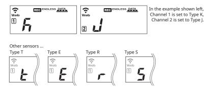
The factory default setting is "K" for both 1 2. Depending on the thermocouple type you're going to use, make settings or changes using "T&D WebStorage Service" or the software "TR-7wb/nw for Windows".
