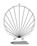
Sensor with No.0207XXXX Broken line: cos θ Solid line: Measurement Values
