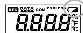
Battery Warning Mark
