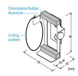
Compatible Device: RTR500BC (Discontinued: RTR-500) Included Items: O-Ring, Lock Screws, Double-Sided Adhesive Tape
