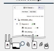
When used in conjunction with Repeaters, the Base Unit will automatically select the best route to ensure stable wireless communication with less errors.
