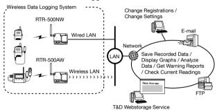
After having registered an RTR-500NW/500AW as a Base Unit and making various settings, the Unit will automatically carry out a series of actions according to settings.
