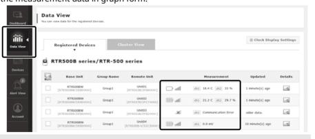
The signal strength between Base Unit and Remote Unit can be checked by color and number of antennas. When using Repeaters, the signal strength displayed here is only that for between the Remote Unit and the nearest Repeater. To check the signal strength between the Base Unit and Repeater or between Repeaters, please use the RTR500BW Settings Utility or T&D 500B Utility.
